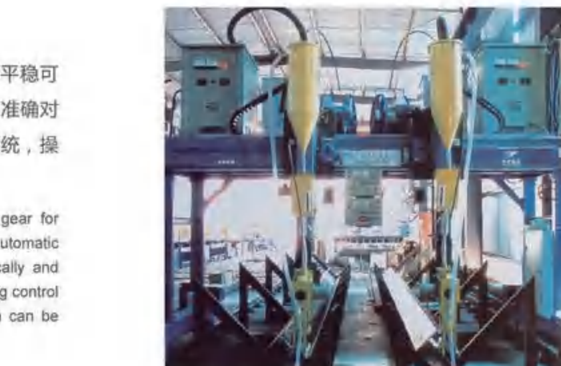
集中控制的龙门焊 Centrally controlled gantry welding
